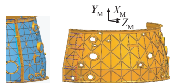
图 10 纵向安装边铣削、钻铰孔和刀路轨迹示意图 Fig.10 Schematic diagram of longitudinal mounting edge milling, drilling and reaming and tool path
